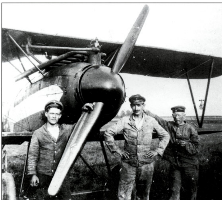
This view provides a good look at the nose of the Kempf/Prien D III and the forward portion of the arrow insignia. Note the cooling louvres cut into the cowling just aft of the spinner and the anemometer-type ASI mounted on the port interplane strut (Prien album)
